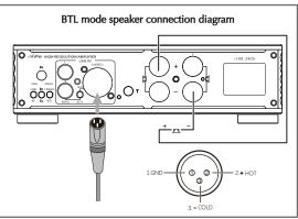
Refer to the BTL mode speaker connection diagram, and connect the passive subwoofer and power supply.
